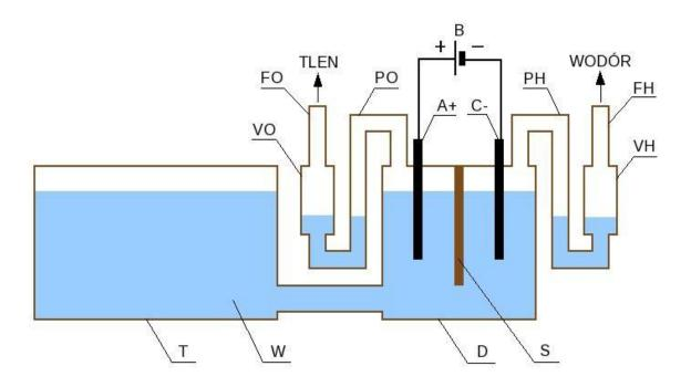
Fig. #C1: The design and main components of the conventional dissociator for the "car on water" - courtesy Szod. (Click on the above drawing to see it enlarged or to shift it to a different area of the screen.)
