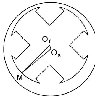
Fig. 1. Positions of rotor and stator air-gap dynamic eccentricity.
