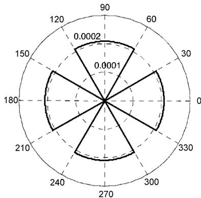
Fig. 3. Polar distribution of air-gap magnetic permeance of a healthy synchronous machine.
