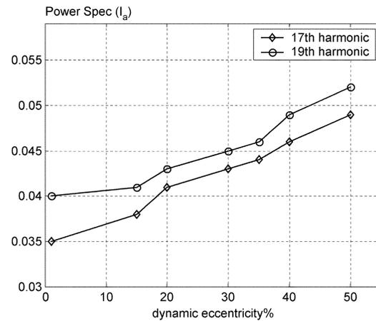
Fig. 13. Amplitude versus eccentricity level for the 17th and 19th harmonics.
