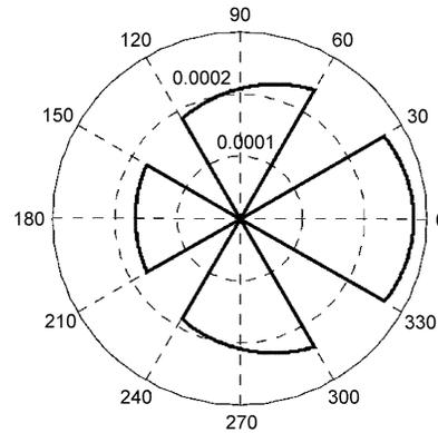
Fig. 4. Polar distribution of air-gap magnetic permeance of a synchronous machine with 25% dynamic eccentricity.
