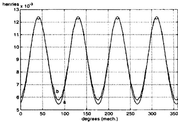
Fig. 11. Calculated self-inductance of phase a of stator with 25% dynamic eccentricity: (a) Unmodified and (b) modified winding function.
