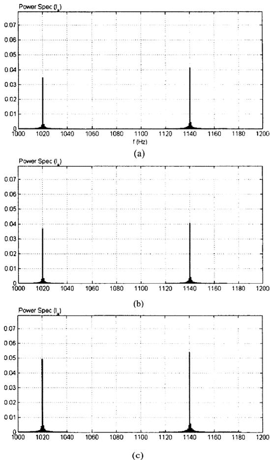
Fig. 12. Frequency spectrum of stator phase current (17th and 19th harmonics) for: (a) healthy machine, (b) 15% dynamic eccentricity, (c) 25% dynamic eccentricity.
