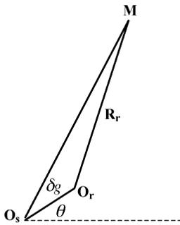
Fig. 2. Position of a point on the rotor pole shoes during air-gap dynamic eccentricity.
