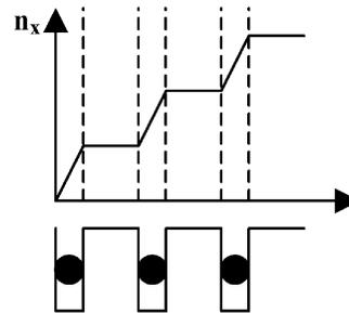
Fig. 5. Turn function of a winding with mmf rise across the slots.
