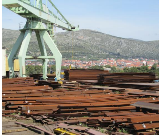
Figure 1: Storage area of plates, profiles and flats in a shipyard
