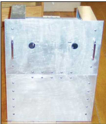
Fig 8—Views of the amplifier module mounted into a chassis for additional testing.
