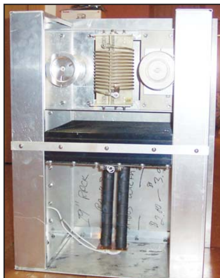
Fig 8—Views of the amplifier module mounted into a chassis for additional testing.
