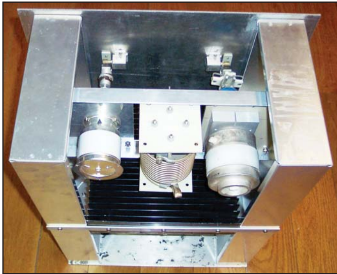
Fig 7—A view of the amplifier module mounted into a chassis for additional testing.
