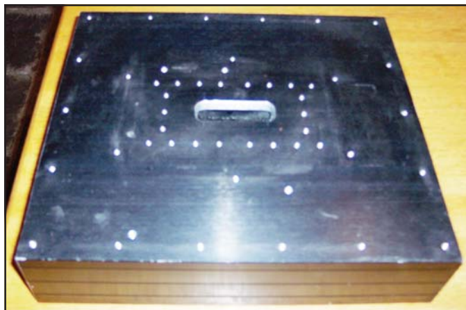
Fig 1—Heat sink with slot and tapped holes for mounting the PC board and components.
