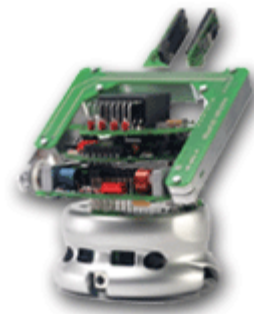
Fig – Khepera II robot
