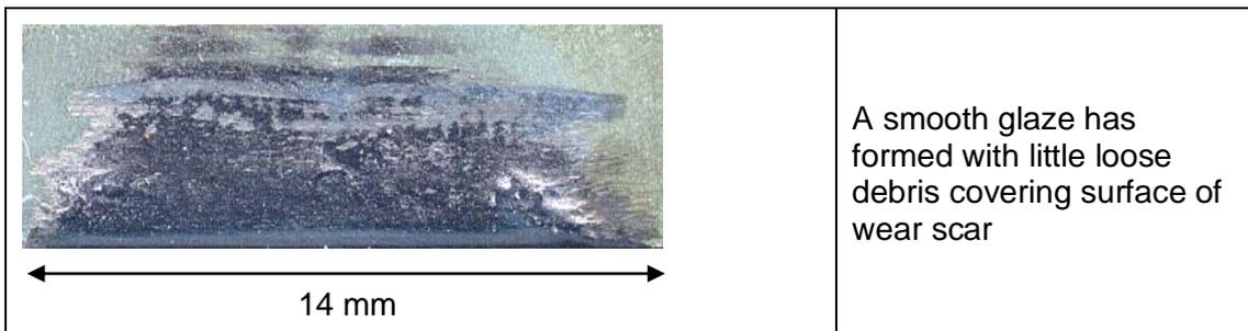
**Figure 5.C4: Compacted oxide produced on Stellite 6 samples slid against a Incoloy MA956 counterface at  $0.314 \text{ m.s}^{-1}$  – SEM images**
