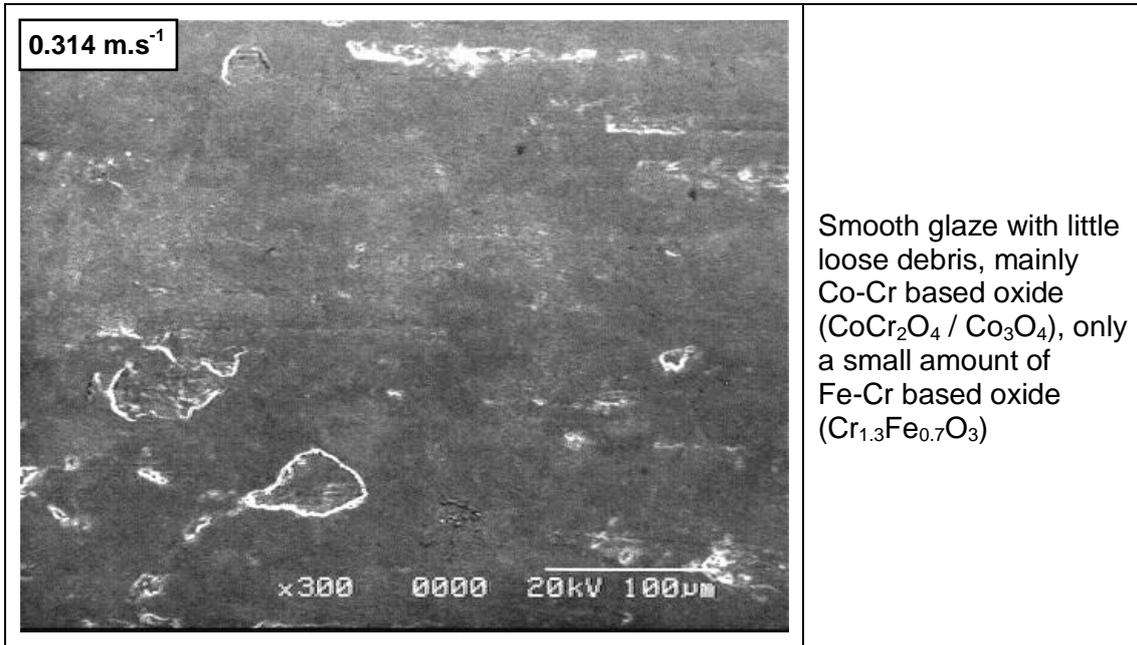
**Figure 5.C5: Backscatter image of the side profile of a Stellite 6 sample slid against Incoloy MA956 at  $0.314 \text{ m.s}^{-1}$**
