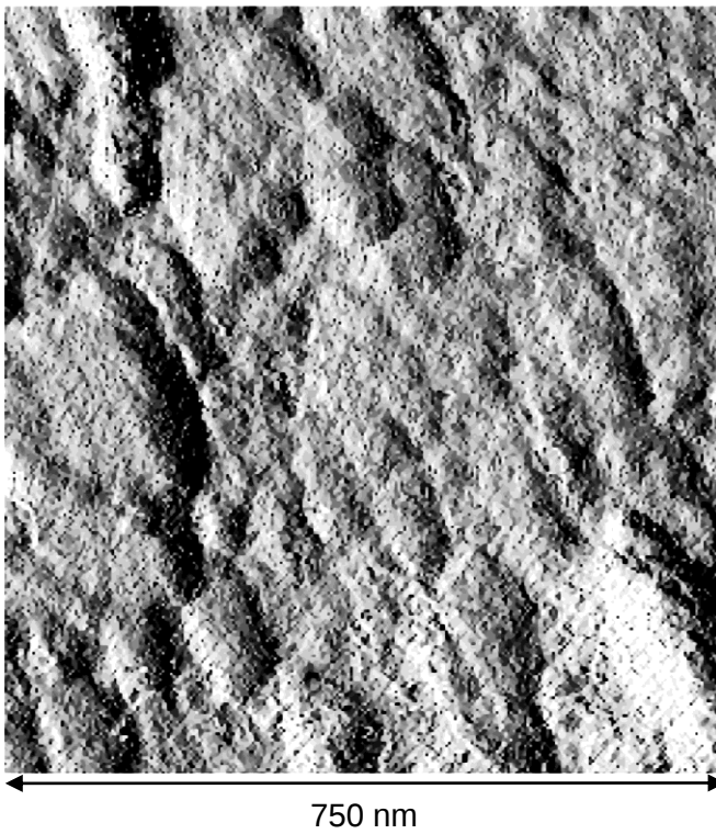
Fig. 4: Top-down AFM image of 'glaze' layer surface produced on Incoloy MA956 at 0.314 \text{ m.s}^{-1} and 750^\circ\text{C}
