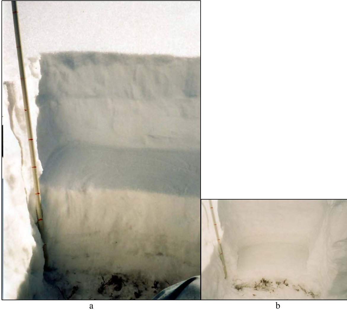
fig 2: view of the profile at different times of collection, a: not compacted snow, b: compacted, icy snow
