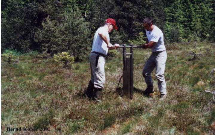
fig 3: The Wardnaar corer is pushed down in the peat.
