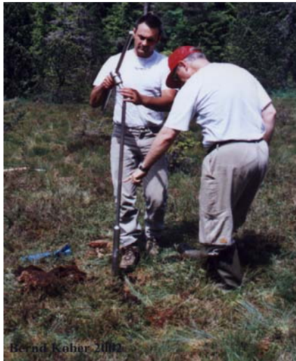
fig 5: The Stainless steel Belarus corer is pushed down alternatively in a second hole and in the first hole done by the Wardnaar corer.
