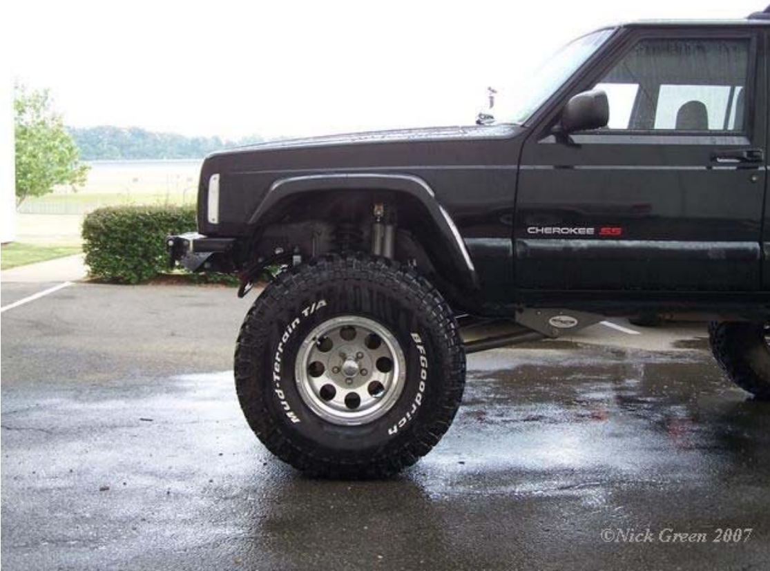
Room with new trimming. These are 35x12.50 tires on a 15x8" wheel with about 6" of lift. Your results will vary based on lift/tires/wheel/trimming combo.
