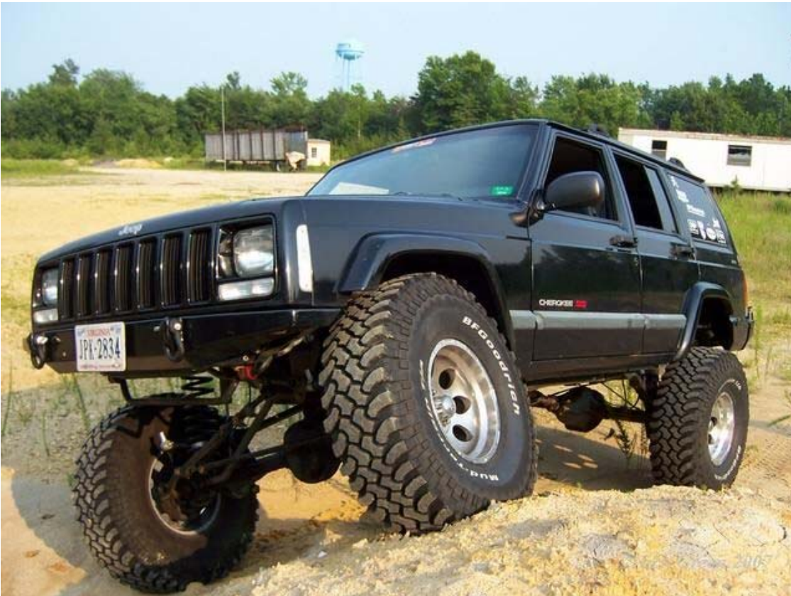
Room with new trimming. These are 35x12.50 tires on a 15x8" wheel with about 6" of lift. Your results will vary based on lift/tires/wheel/trimming combo.
