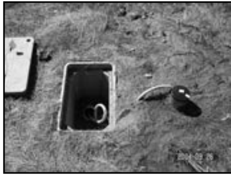
The UCLA magnetometer is buried in the ground.
