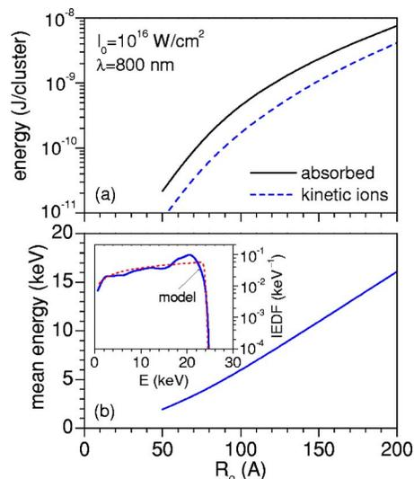
FIG. 2. (Color online) Absorbed energy per cluster (solid line) and energy converted into kinetic energy of ions (dashed line) vs initial cluster radius (a), and mean ion energy vs initial cluster radius (b). The inset in (b) shows the IEDF for  $R_0 = 200 \text{ \AA}$ . Peak laser intensity:  $I_0 = 1 \times 10^{16} \text{ W/cm}^2$ ; wavelength:  $\lambda = 800 \text{ nm}$ ; pulse duration:  $T = 400 \text{ fs}$  (150 laser cycles).
