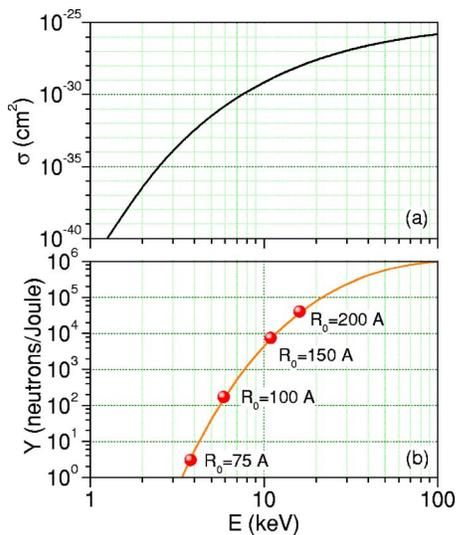
FIG. 3. (Color online) Cross section for fusion reaction  $D+D \xrightarrow{50\%} He^3+n$  (a), and neutron yield vs  $D^+$  kinetic energy for laser energy  $E_{\text{laser}}=1$  J and target with density  $N_D \sim 2 \times 10^{22}$  cm<sup>-3</sup> and thickness  $L=1$   $\mu\text{m}$  (b). Yield for clusters with an initial radius of 75, 100, 150, and 200 Å.
