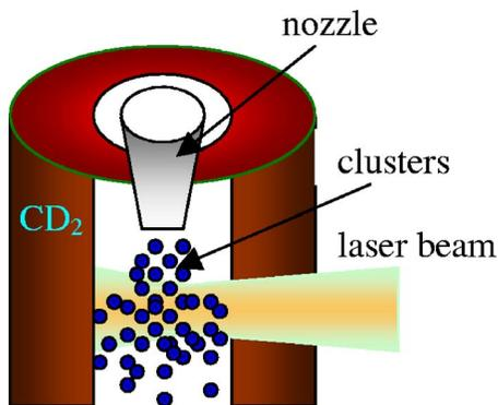
FIG. 1. (Color online) Schematic diagram of the reaction chamber. The target material is  $\text{CD}_2$  with thickness 1 mm.
