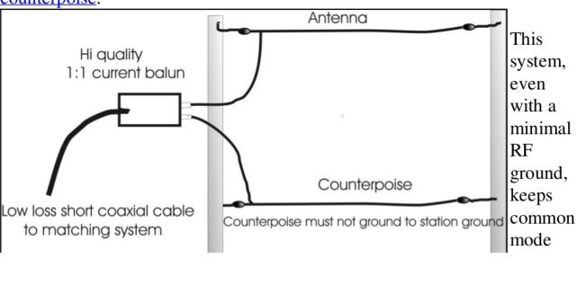
out of the operating area. This system reduces noise and RFI. It generally eliminates the need for a shack "floor groundplane". The balun must be a reliable current balun with high common mode impedance. A voltage balun, or a single core 4:1 balun, will make things worse.
