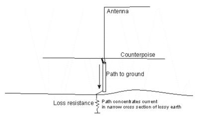
The **Counterpoise wire** runs down from the 17' pole, then along the brick side of the house, and attaches to the back fence, ungrounded. My counter-poise is about 20' long, and not grounded at the antenna. Ideally it would be a few feet of the ground, but mine is 10' up, 20' long.
