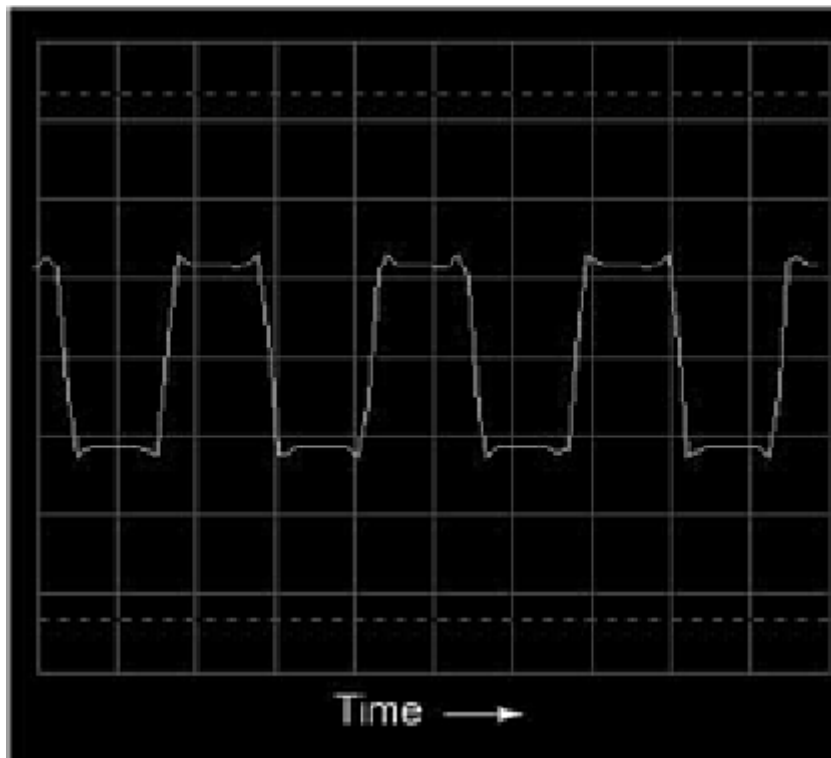
Oscilloscope time-domain display of a square wave
