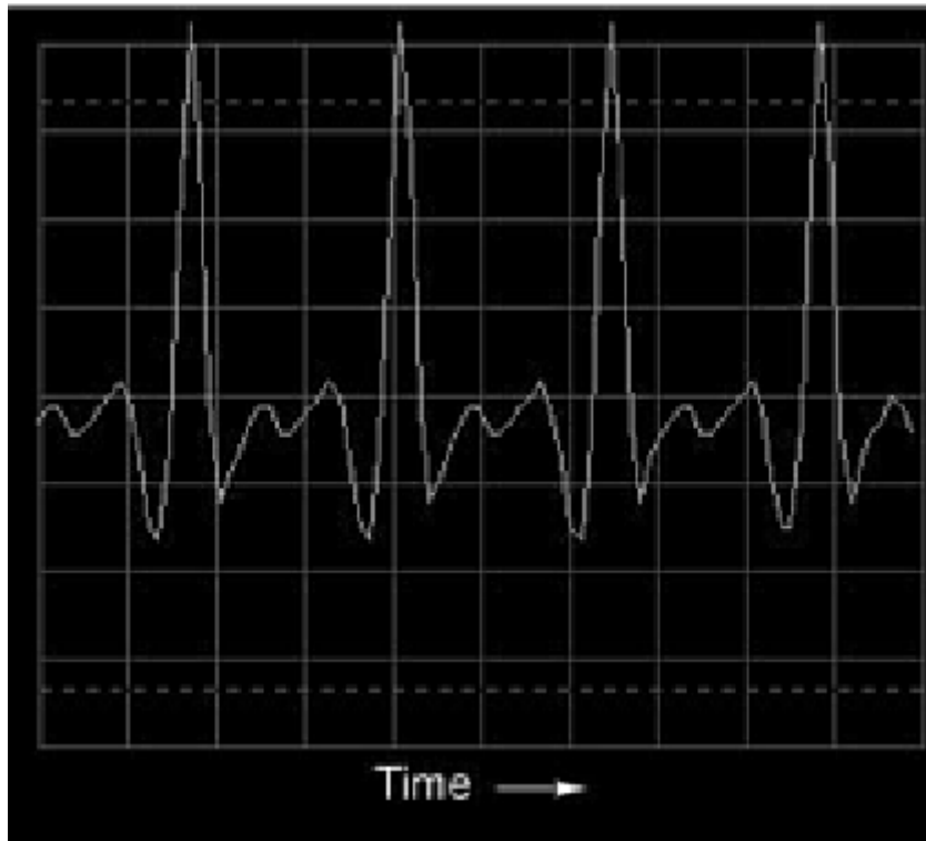
Oscilloscope display: waveshape of a trumpet tone.
