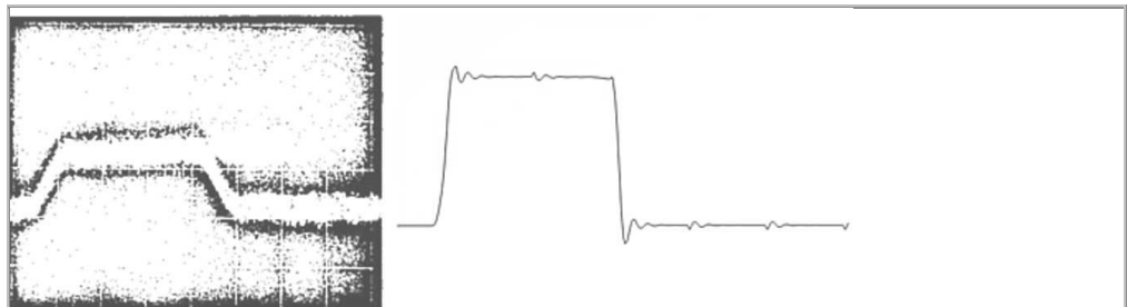
Figure 12. Pulse details buried in a noisy screen display are clearly revealed using rate-adaptive scanning.
