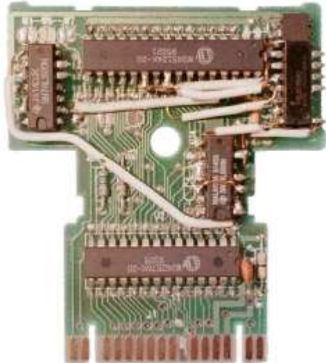
Figure 3 Completed Dev Cart using two 64Kx8 SRAMs
