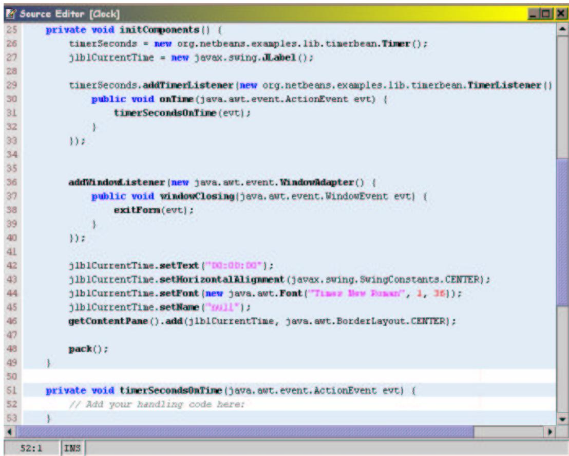
The screenshot shows the NetBeans IDE interface with a source editor titled "Source Editor [Clock]". The code is written in Java and defines a class named "Clock". The code includes methods for initializing components, handling window closing, and updating a label with the current time. A placeholder comment "// Add your handling code here;" is present in the timer handler. The status bar at the bottom shows "52:1" and "INS".
