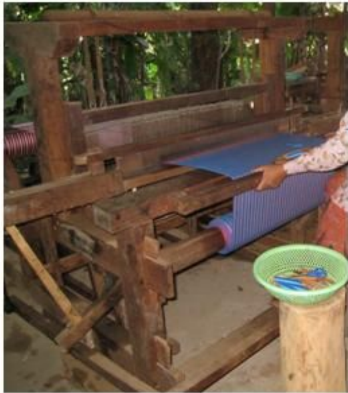
1. Different color threads are manually slot on the weaving machine
