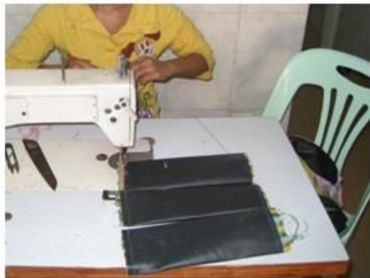
6. Inner lining is sewn together with the weaved fabric
