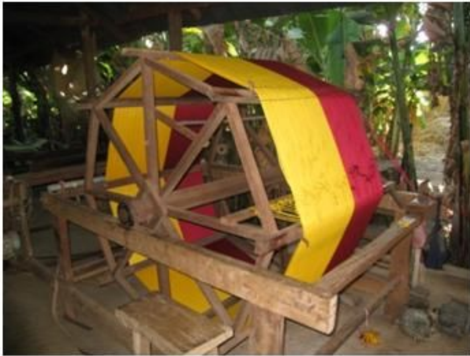
1. Thread are coiled manually onto roller
