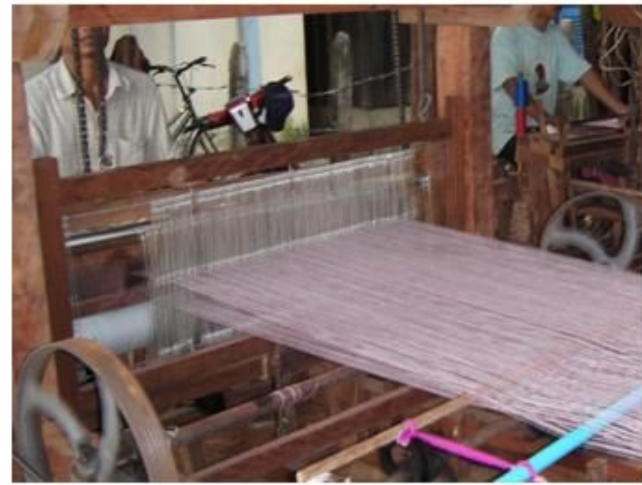
2. Worker has to put the thread into layers before starting the weaving process
