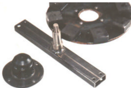
Spine, shaft, hub and magnet rotor
