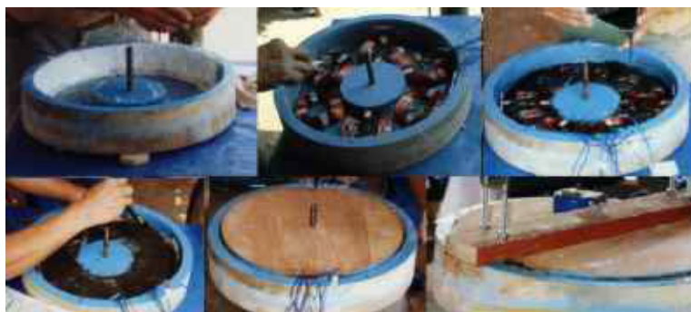
Six stages of the rotor casting procedure
