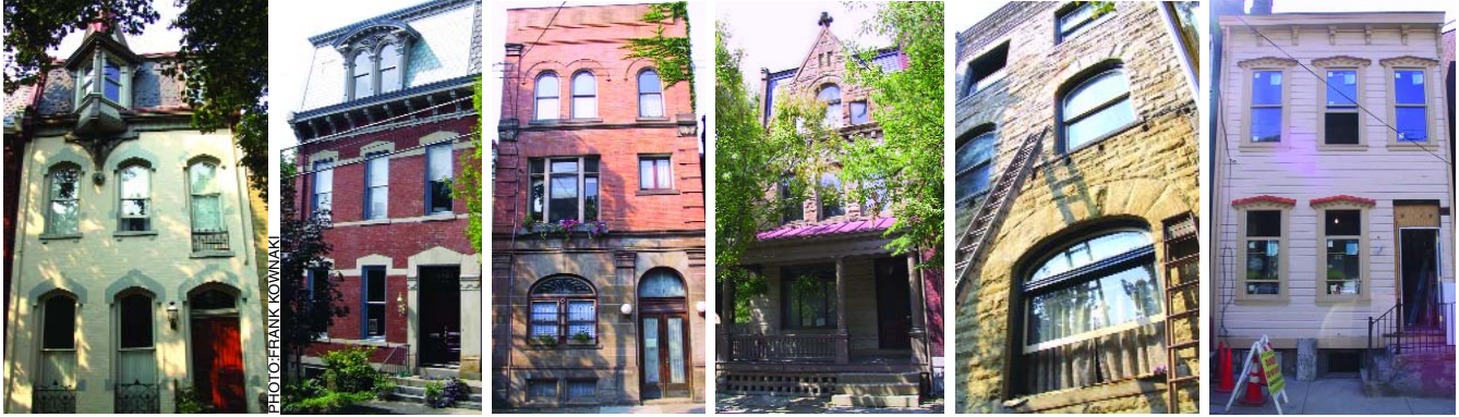
Left to right: One of the few true Gothic Revivals defined by its pointed arches of the window hoods and the gothic embellishments of the turret; This Second Empire has the distinctive mansard roof and arched dormer; Typical of the War Streets, a structure often had a mix of styles i.e. Richardson first floor, Italianate on the second floor, and Second Empire on the third; This restored Richardsonian Romanesque brackets the Richardson row on Buena Vista and was the parsonage to what was once the Westminster Presbyterian Church across the street; Another member of the Richardson row is undergoing a total renovation; An example of the earlier vernacular wood frame houses undergoes a gut-job and facelift.
