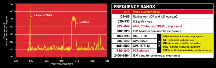
**CELLULAR STANDS OUT:** The wideband signal on the right side of the graph is a CDMA signal (CDMA channel 466). The narrowband signal on the left is likely either an analog or a TDMA signal. The wideband signal's weaker appearance is due in part to the settings of the measuring equipment.
