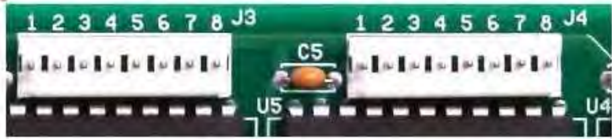
Cable header for connection to graphic annunciator's On/Off LEDs (J3 = Groups 1-4; J4 = Groups 5-8)
