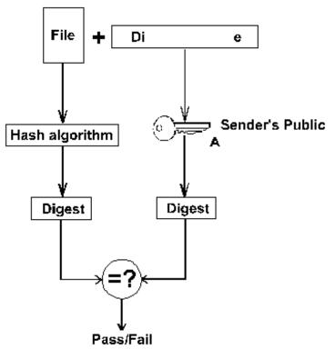
This diagram shows process at receiver's end to check the signature after the message has been decrypted
