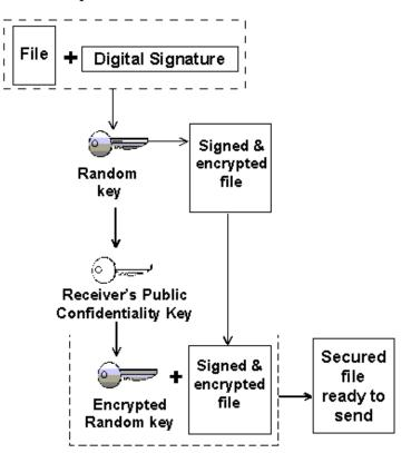
This diagram illustrates the process of encryption
