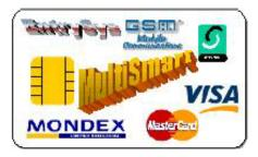
An imaginary multifunction smart card, including GSM SIM; credit, debit and cash card; and entry control functions
