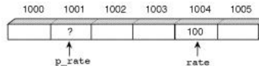
Figure 9-2. Memory storage space has been allocated for the variable p_rate .
