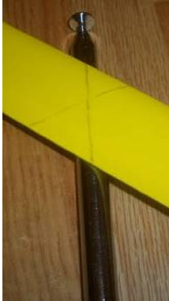
Figure 12: Finding Center of Gravity for Blade 1
