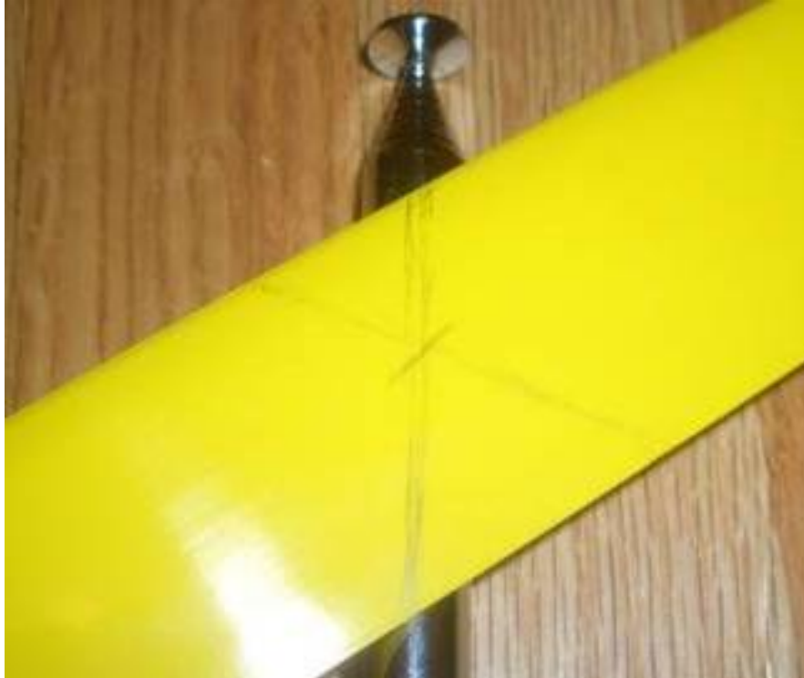
Figure 13: Finding Center of Gravity for Blade 2
