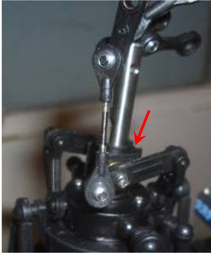
Figure 8: Shaft Sliding Set
