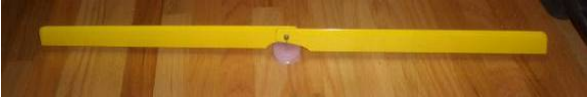
Figure 16: Blades Balancing on Needle Stand
