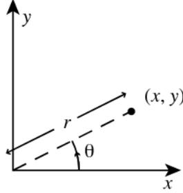
$$\det(J_\varphi(r, \theta)) = \begin{vmatrix} \frac{\partial x}{\partial r} & \frac{\partial x}{\partial \theta} \\ \frac{\partial y}{\partial r} & \frac{\partial y}{\partial \theta} \end{vmatrix} = \begin{vmatrix} \cos \theta & -r \sin \theta \\ \sin \theta & r \cos \theta \end{vmatrix} = r \cos^2 \theta + r \sin^2 \theta = r \neq 0.$$
