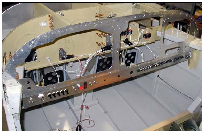
Warren's RV-6 in the wiring stage
