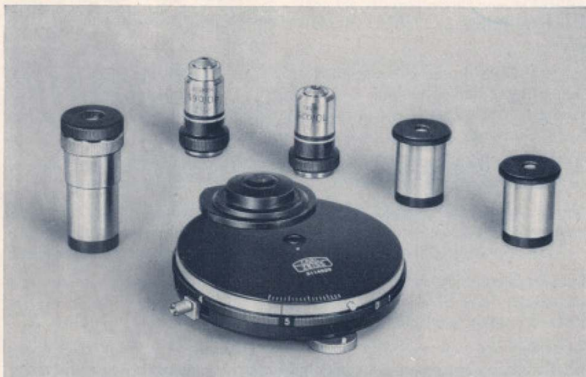
Fig. 21: Bright-field, phase-contrast, dark-field condenser III Z 6 with centering telescope (left), phase-contrast objectives, and C-eyepieces.
