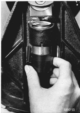
Fig. 3 Removing the lamp condenser from the microscope stand
