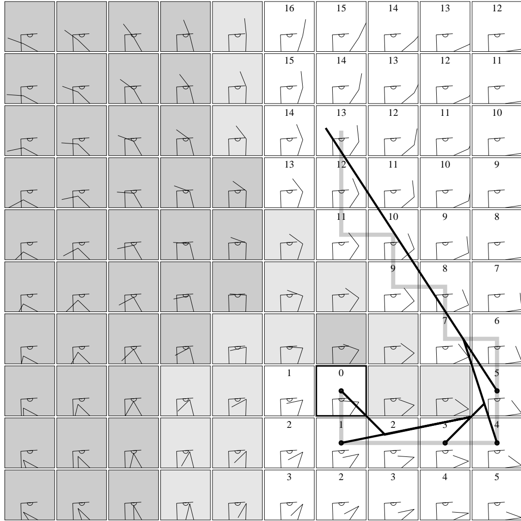
Figure 4. A two-dimensional slice of the configuration space map. Cells approximating safe, near-colliding, and unsafe regions are shaded light, medium, and dark gray. A goal cell representing a self-touching posture is highlighted with heavy black outline. Cells are drawn with their corresponding postures. Each safe cell is labeled with the value of the NF1 potential, which measures the distance around the unsafe region to the nearest goal cell. The thick gray line is an example NF1 gradient descent path, and the black lines represent the corresponding smoothed path. Terminating extensions off the smoothed path represent intermediate points p^I ; the last terminating extension represents the final goal point p^G . In most cases, the path changes direction before reaching an intermediate point. Although the two-dimensional path depicted here represents the movement of only the right arm, in general the four-dimensional path represents both arms moving simultaneously.
