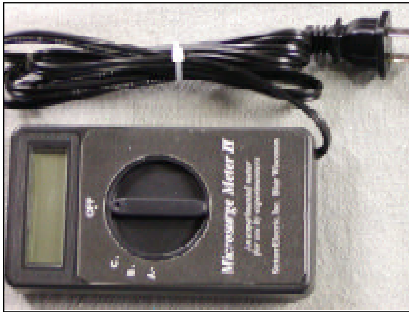
This inexpensive meter developed by Dr. Martin Graham detects levels of radio-frequency radiation on household wiring.
