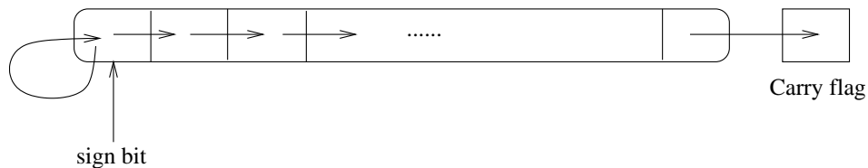
Figure 6.5: Arithmetic right shift
