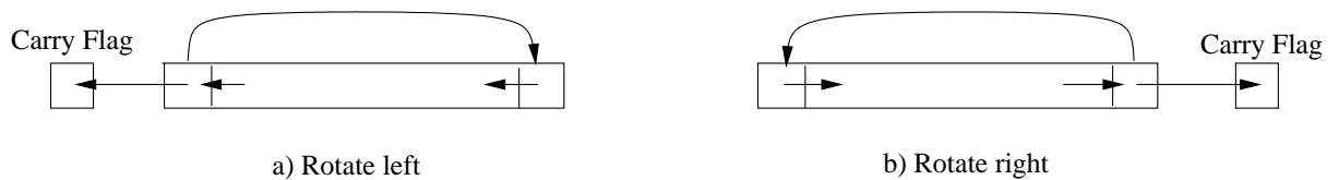
Figure 6.6: Rotate shifts
