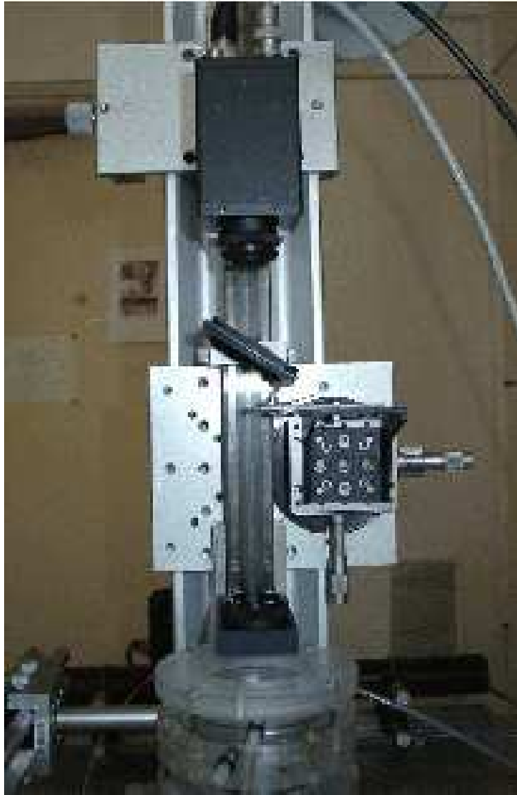
Figure 4.8: A view of the Schlieren system. From the bottom, we see the cell, the focusing lens, the blade, held by a micrometric mount, the neutral filter and the CCD camera.
