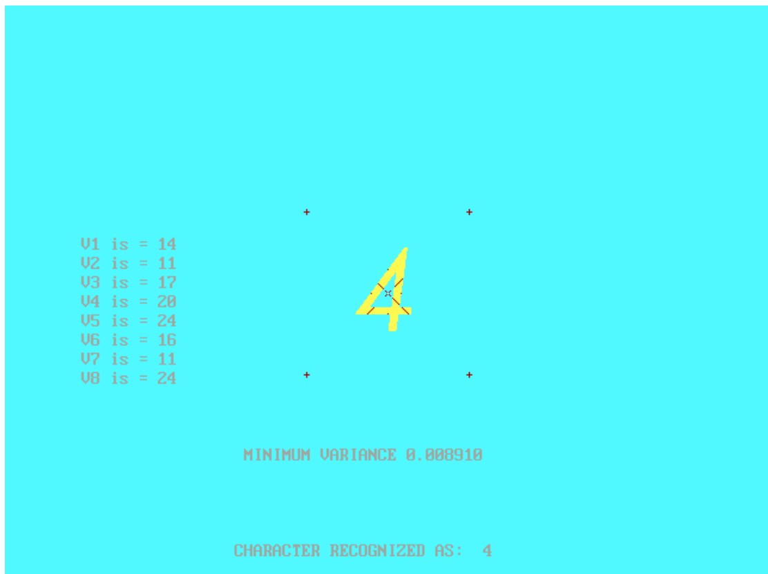
FIG 16 :CALCULATING VARIANCE AND DISPLAYING RECOGNITION RESULTS.
