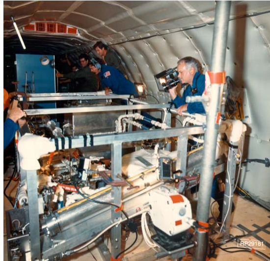
FIGURE 5. KC-135 Flight Test. Clear Shear Flow Condenser in Foreground.
