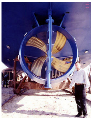
Figure 1.5. Rear view of a Kort nozzle (ducted propeller) with single rudder. (Olds, 2006)
