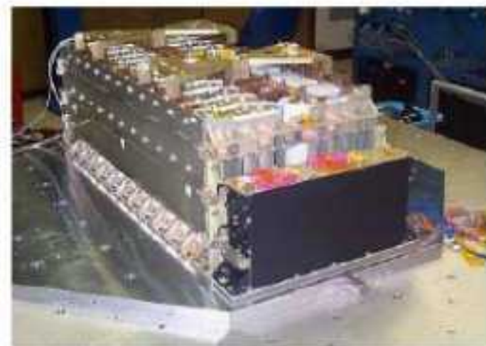
24-Cell Battery Assembly
