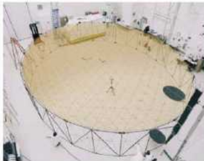
ASTRO 12m MBSat Reflector
