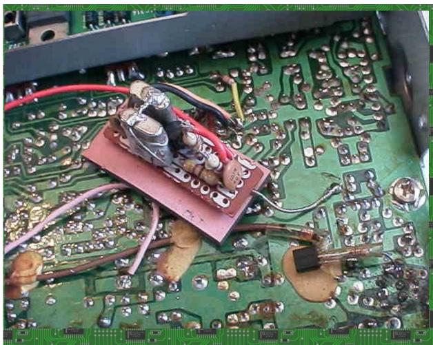
Power is taken from the + lead where it is soldered the the main board. But it can be on the power switch where it would be off when the radio is off. The ground can be made to the large trace and solid tinned wire will allow the filter board to be secure.
