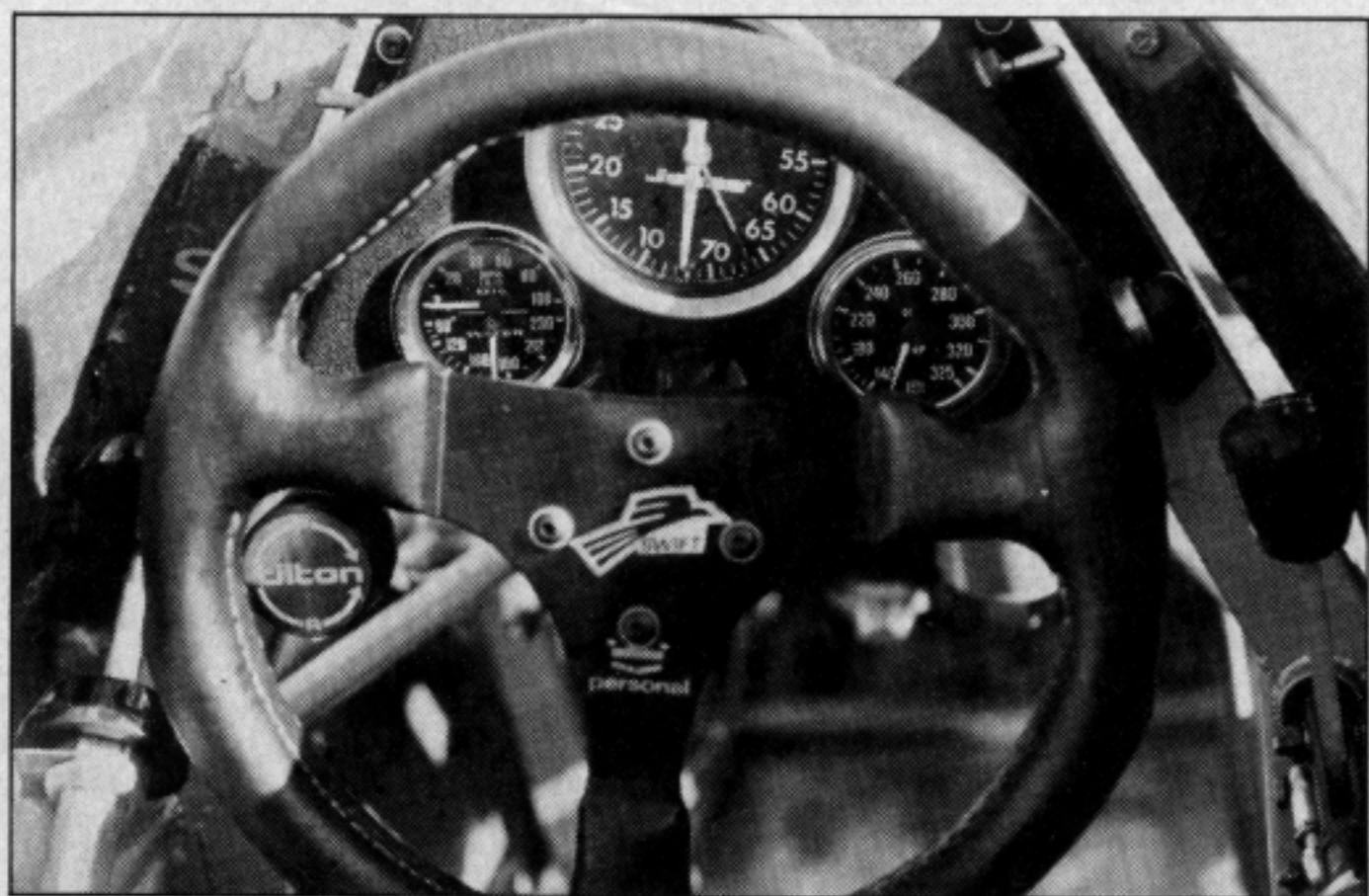
Only the essentials occupy valuable dashboard real estate. Control for rear anti-roll bar adjustment is visible at left, as is knob for fore/aft brake balance.
