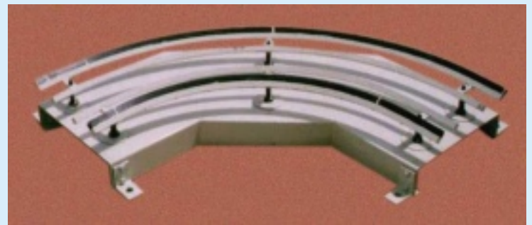
Line Turning Device For 90 Degree turning of glazing
