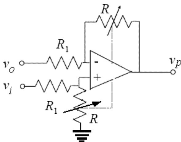
$$V_p(s) = \frac{R}{R_1}(V_i(s) - V_o(s)) = \frac{R}{R_1}V_e(s)$$
