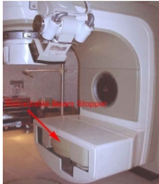
Figure 1-3. A beam stopper incorporated in a linear accelerator 12 .
