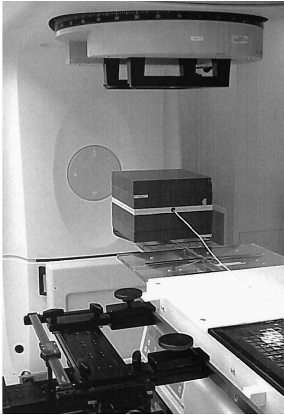
Fig 10. Dose validation by performing absolute dose measurements using a 0.125-cc chamber in standard 30 \times 30 \times 22 -cm phantom.
