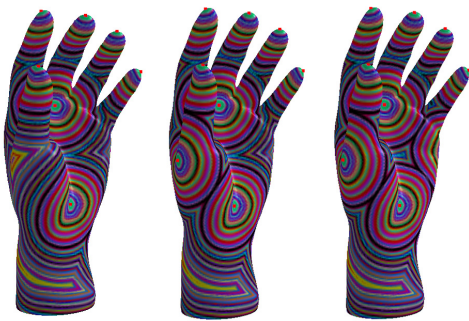
Figure 1: Wave propagation for the incremental computation of geodesic Voronoi diagrams and thus progressive intrinsic (red) farthest sample point localisation of 10, 11 and 12 sample sites on a triangulated surface (from left to right).
