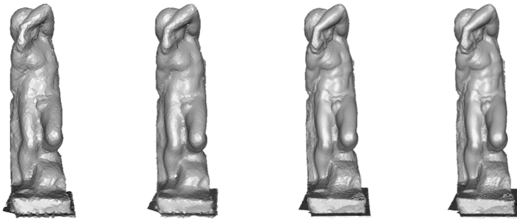
Figure 9: Examples for the quality of the point distributions generated by our algorithm: The Michelangelo Day (left) and Dawn (right) data sets uniformly subsampled to 1% of their original size and their corresponding surface reconstructions. (This Figure is best viewed on-screen).
