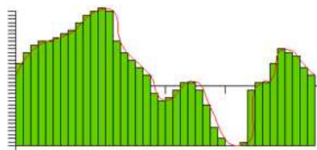
An analog-to-digital converter measures sound waves at frequent intervals.
