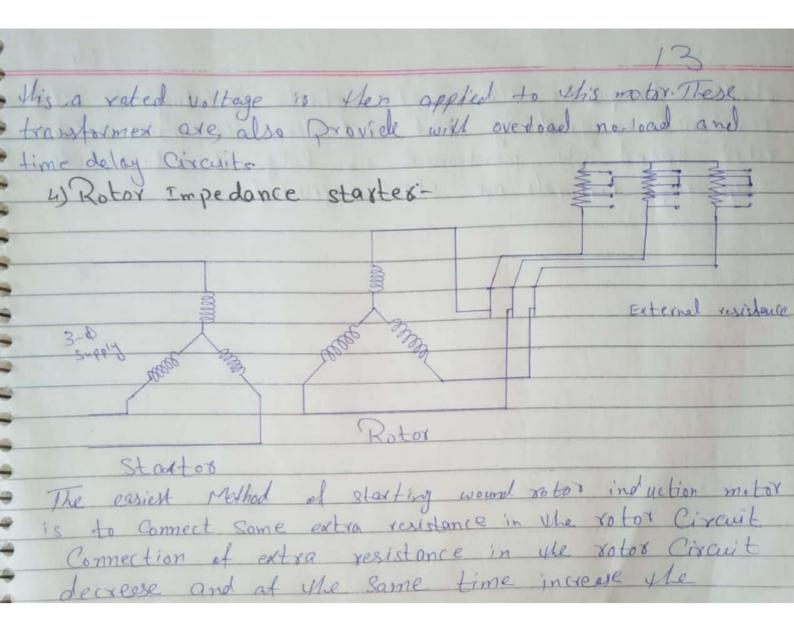
Starting tryque. As the motor starts rotating the extre resistance is gradually out out when the motor estains rated speed the resistance is fully out out and the slip ring terminals are short circuited.
