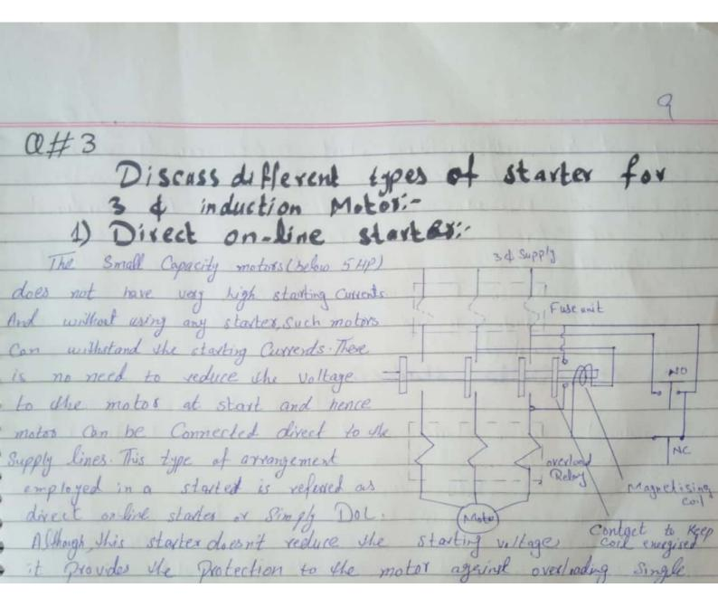
Plasing and low voltage. During start condition normally appear Conduct is pushed for fraction of a Second and this makes the magnetising coil becomes energised. This magnetic flux produced by the Coil attracts the Contactor so that the motor is now Connected to the Supply when a Ad C. Switch is pressed. The Coil becomes de-energised and the Conductor get separated by spring arrangement there by the Supply to the motor is removed.
