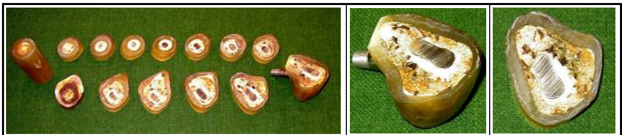
Figure 2.14: Transverse sections of an impaction grafted Sawbone ® femur indicating the geometry of the biomechanical problem.
