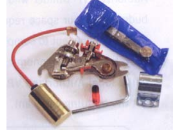
This points and condenser set came with everything needed to do the job, including the small tube of distributor cam lube. Over the counter price was $14.99.
