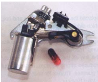
The points and condenser set shown is for a GM vehicle and is referred to as “Unipoints.” As seen here, the condenser is permanently attached to the bracket assembly. This unit retails around $6.99.
