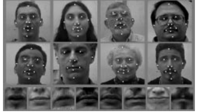
Figure 1: ROI extraction examples. Upper rows : Example video frames from 8 database subjects, with detected facial features superimposed. Lower row : Corresponding extracted mouth regions of interest.
